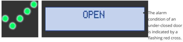
The condition will appear after the timeout of the door closing option 422. In addition, you can use the SW2 output on the power supply to pass this information on (sound or light signal).
